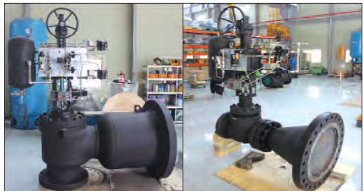
GLOBE CONTROL VALVE ANGLE STEAM VENT
